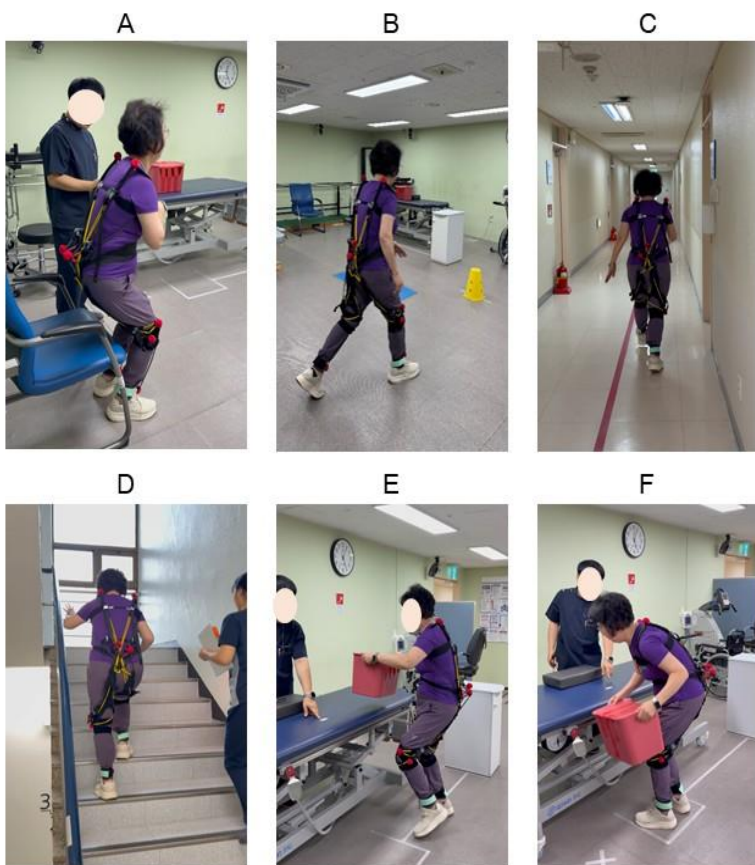
Fig 1. Functional assessments with exo-suit: (A) 30-second chair stand test, (B) Timed up and go test, (C) 6-minute walk test, (D) Stair climbing task, (E) Short carry task, (F) Lifting low task.
