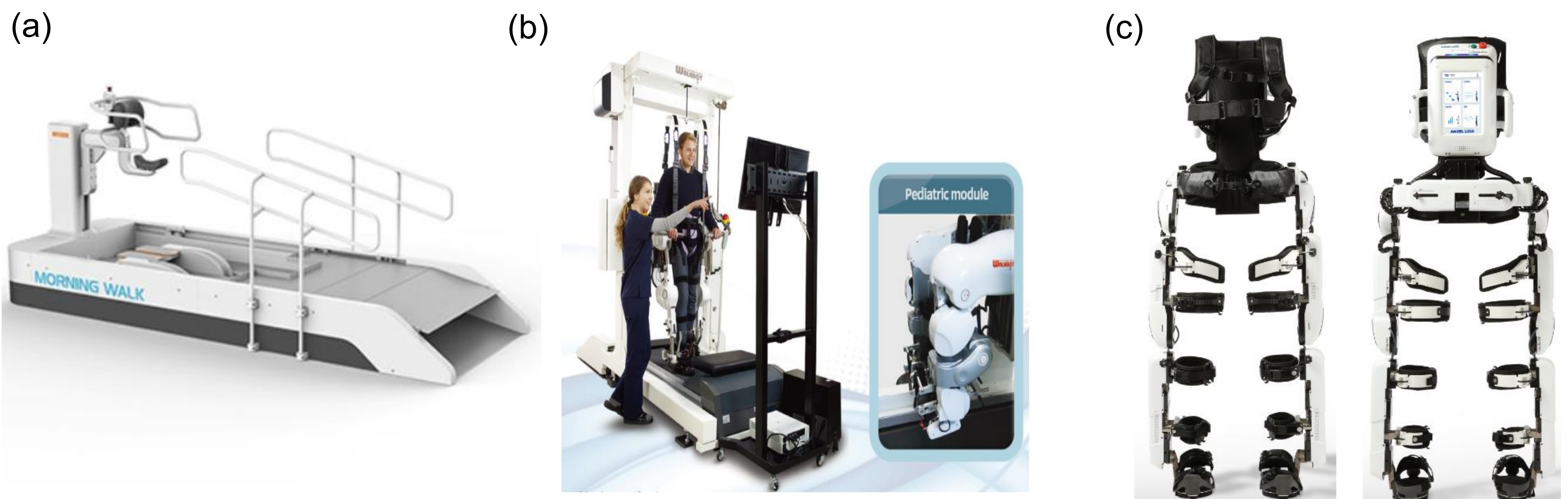
Fig. 1. The gait training robots. (a) Exoskeleton-type Walkbot, (b) End-effector type Morning Walk, (c) Wearable type Angel Legs
