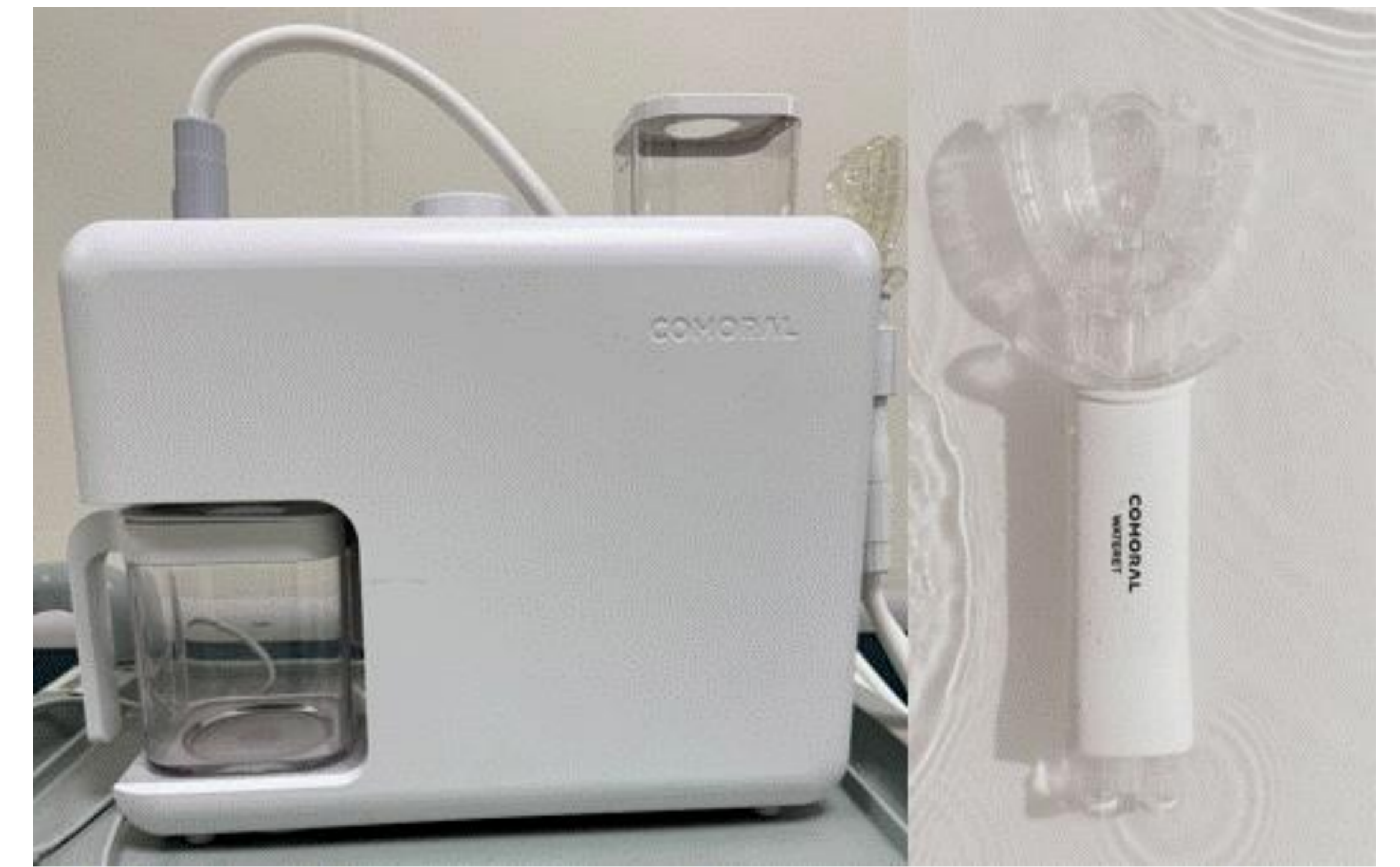
Figure 1. Composition of the multi-channeled oral irrigation device (COMORAL®)
