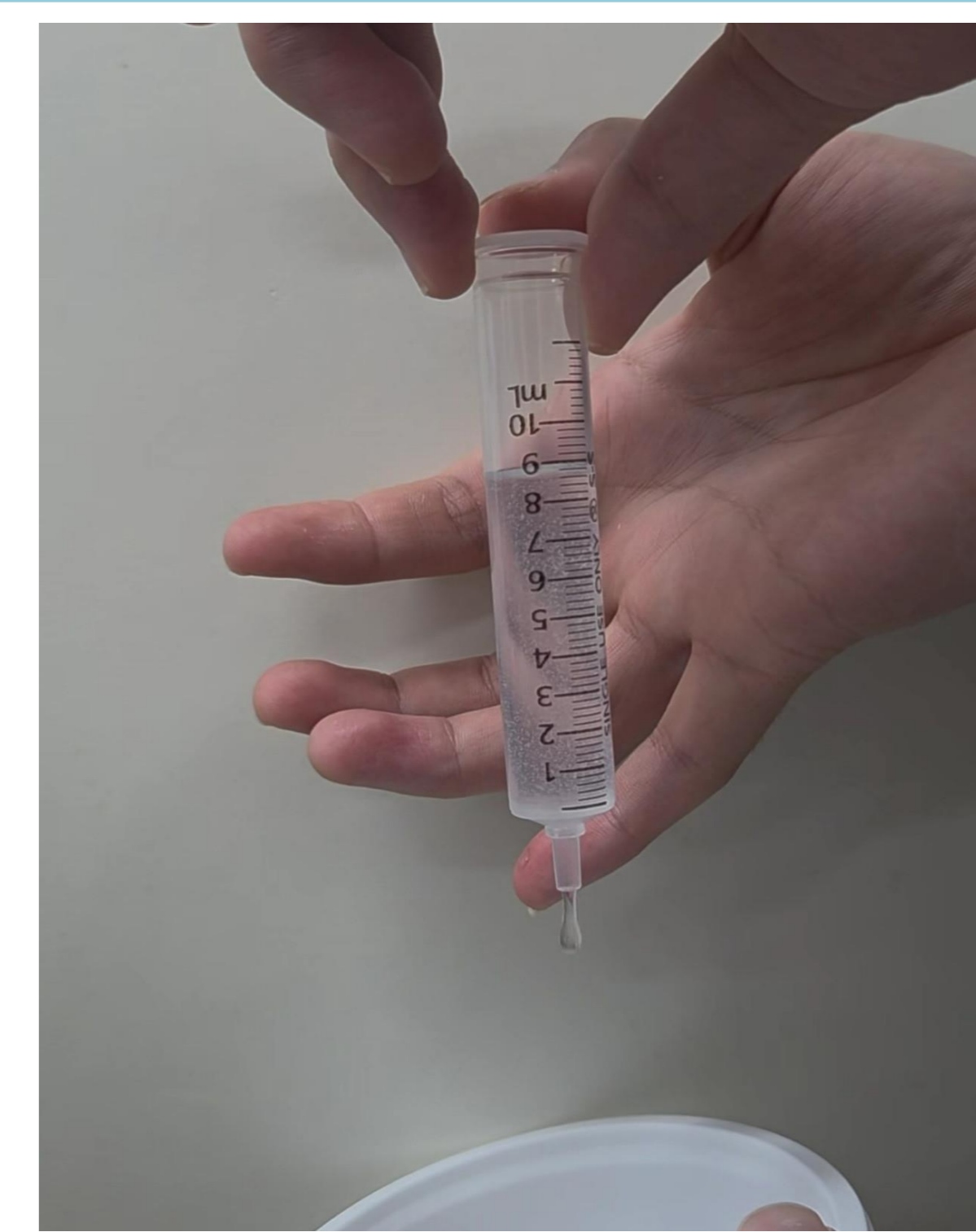
Figure 3. Xanthan gum-thickened water met IDDSI Level 3 by flow test despite relatively low apparent viscosity at the selected shear condition.
