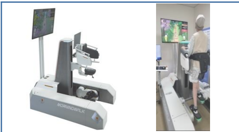
Figure 1. End-effector Type Robot (Morning Walk ® )-assisted Gait Training (RAGT)
